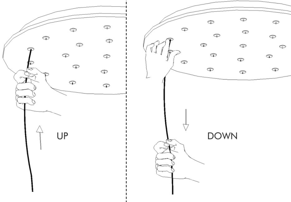
**6** To adjust wire lengths: NEVER TUG ON WIRES! The fixture comes assembled at the maximum length. Lengthening a wire can only be done once it has been shortened. Never try to lengthen wires past the maximum length.
