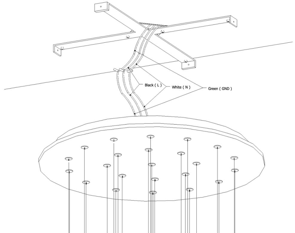
**3** Make the electrical connections to the corresponding wires, then re-attach ceiling mounted bracket to the canopy using provided screws.
