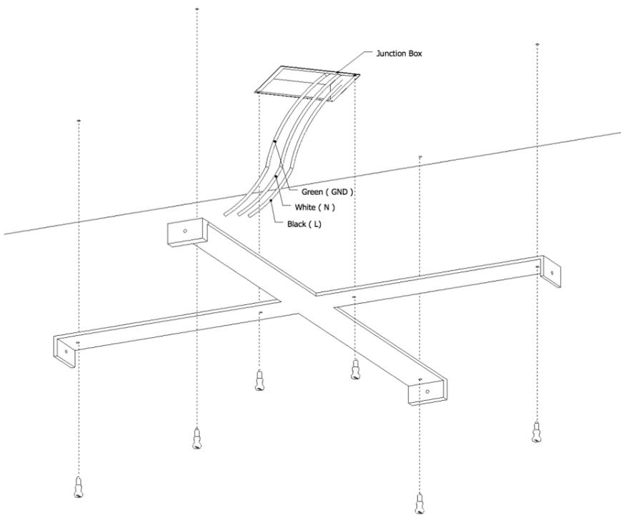
**2** Install the metal bracket to the ceiling using (customer provided) screws, anchors and fasteners.
